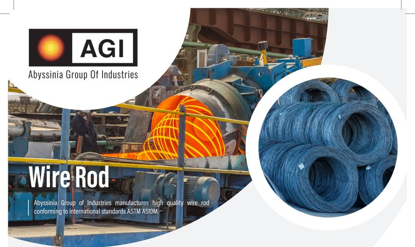
AGI manufactuers and supplies wire rods with nominal diameters from 5.50 mm to 16.0 mm. The rod is rolled from billets into control-cooled coils, yielding a suitable microstructure for subsequent down stream processes. Typical results show the surface defects is less than 1% of the diameter.
